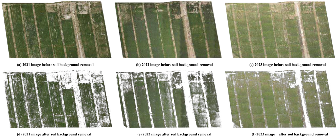
Fig.4 Soil background removal based on Canny edge detection algorithm
