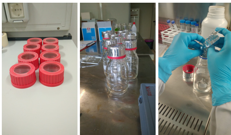
Figure S1: Modified caps of the bottles with the top surface made of quartz (left) and bottles ready to be filled with fibers (center and right).
