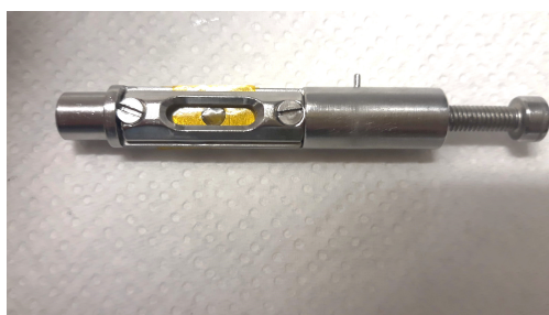
Figure S4: SAXS cell used during the SAXS/WAXS experiment at Elettra in December 2021. The solid sample of the fibers was adjusted inside the cell and then irradiated by X-ray.
