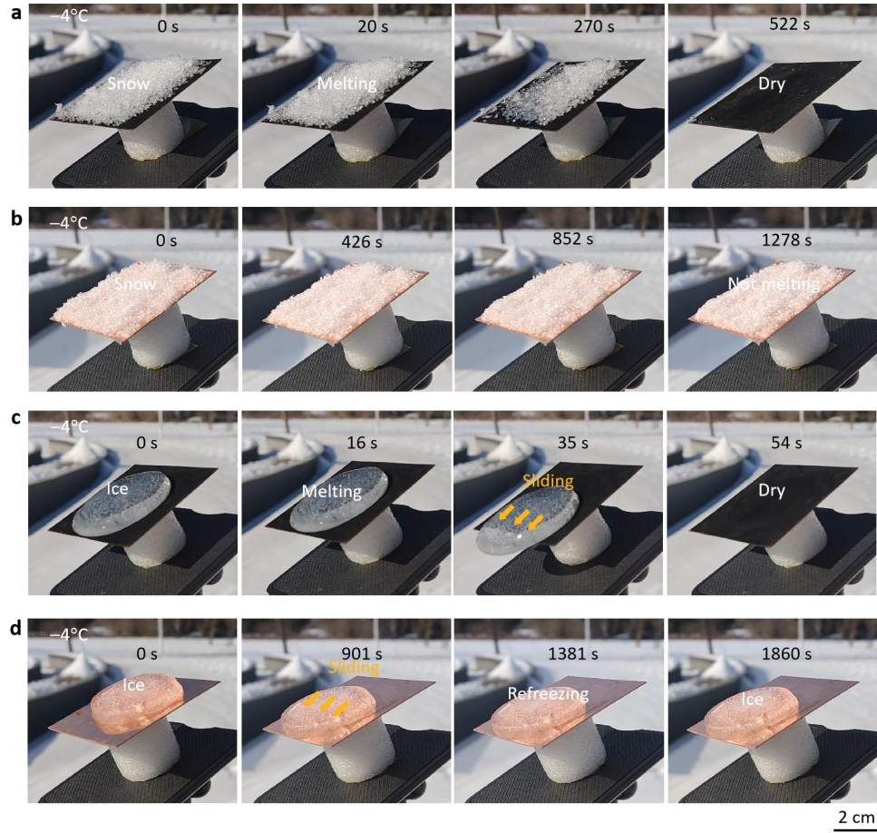
Fig. 20 Outdoor photothermal snow and ice melting performance of IPMM at -4^{\circ}\text{C} . a , Selected snapshots showing the process of photothermal snow melting performance of the IPMM. The snow on the IPMM completely melted after \sim 522 s under sunlight illumination. b , Selected snapshots showing the process of photothermal snow melting performance of the pristine copper surface. Snow isn't melted on pristine copper surface at \sim 1278 s. c , Selected snapshots showing the photothermal deicing process of the IPMM. The ice on the IPMM slides completely down within \sim 54 s under outdoor sun illumination. d , Selected snapshots showing the photothermal deicing process of the pristine copper plate. The ice still exists on the pristine copper plate at \sim 1860 s.
