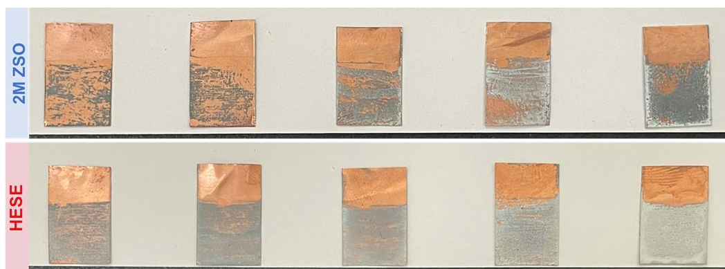
Fig. S25 Digital photographs of the initial nucleation and growth processes of zinc in two electrolytes
