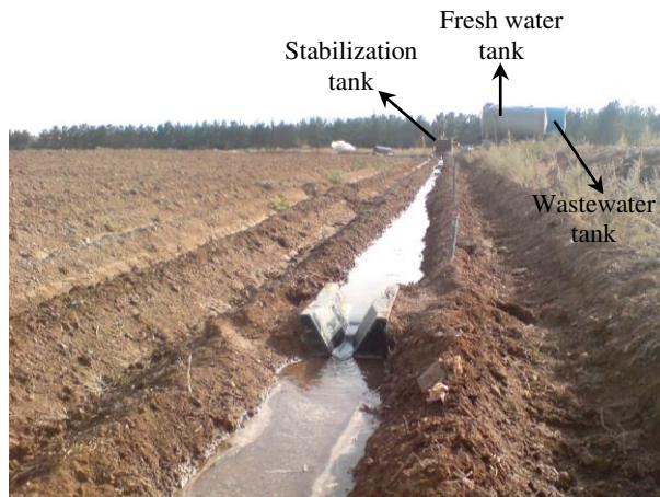
Fig 2. Three tanks and flume used in research (view from furrow end)
