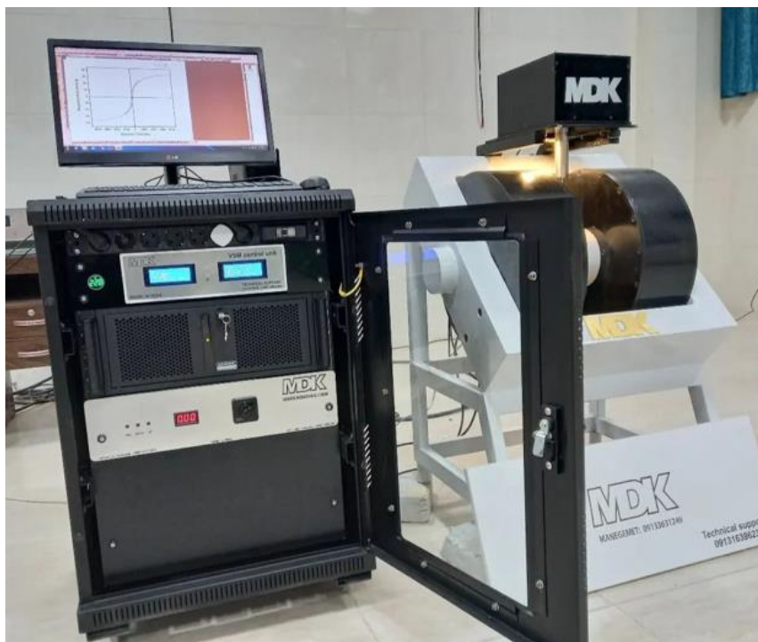
Figure 4: Vibrated Sample Magnetometer (VSM) (MDK-Kashan-Iran) used for magnetometric measurements of this study.
