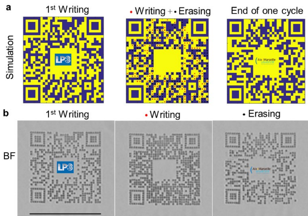
Fig. S7-8. Laser writing of reconfigurable QR codes inside Si a. Simulated QR code points in grayscale format where writing and erasing sequences are described to change the information from the LP3 to the Aix-Marseille University URL. b. Corresponding BF infrared microscopy images of the laser written QR codes inside Si. The scale bar is 100 μm.
