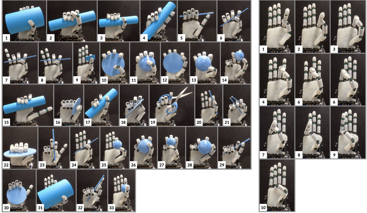
Figure S1. The ADAPT Hand showing all 33 grasp taxonomies and the 10 Kapandji score posture.
