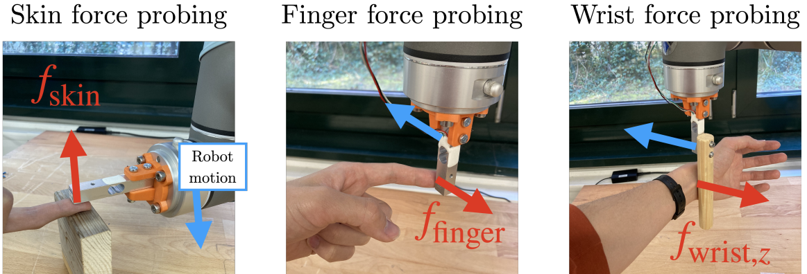
Figure S7. The measurement of human compliance (force-displacement characteristics) using a UR5 robot arm mounted with a 10kg loadcell. The robot arm is moved in different axis to while the human is instructed to relax.
