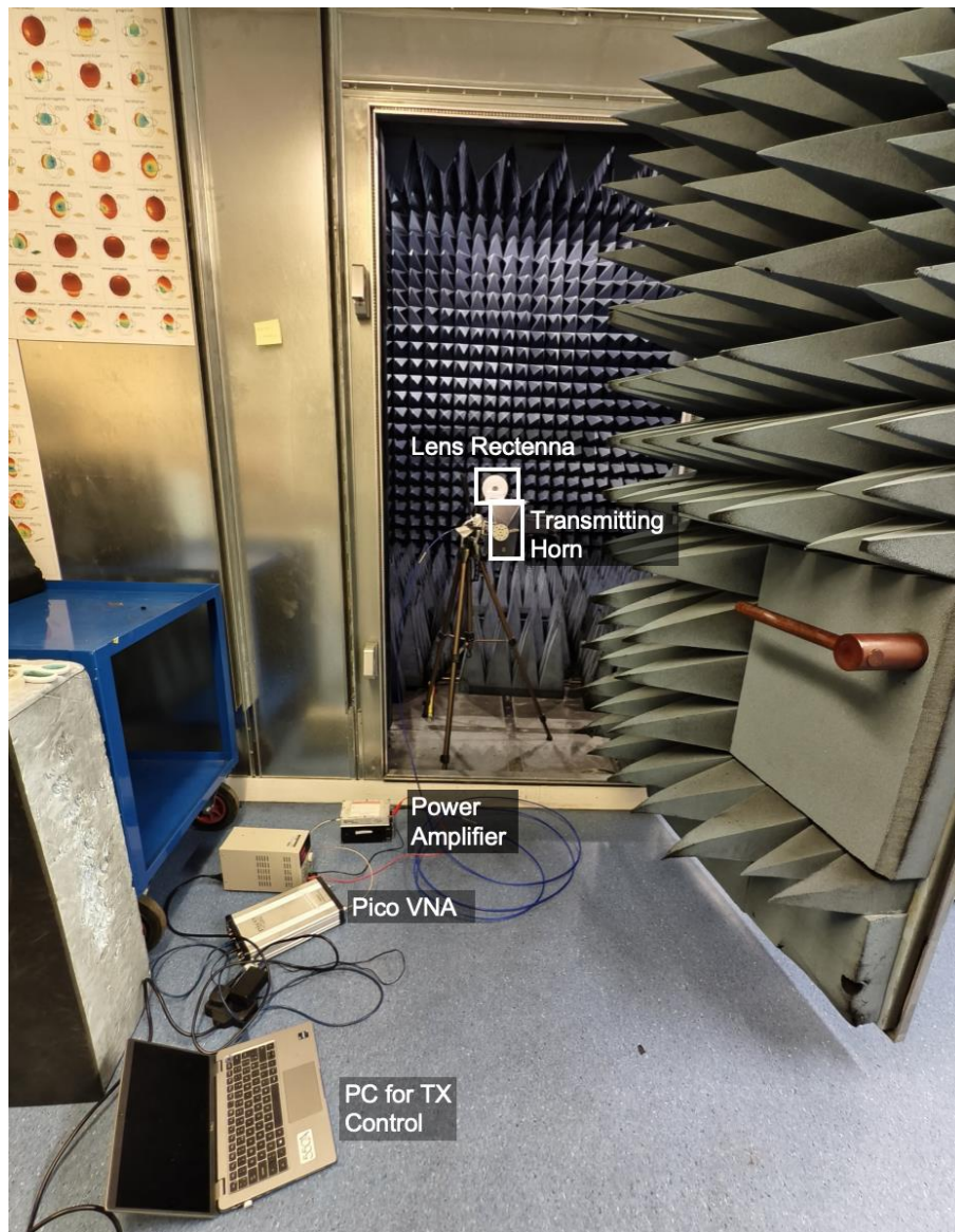
Supplementary Figure 44. Measurement setup of the antenna in an anechoic chamber
