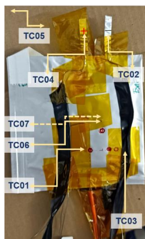
Figure S12. The setup of the multi-layered prismatic pouch cell equipped with the reference electrode, the optical fiber, and seven thermocouples (TC) for the operando WAXS measurement. (a) Back side of the multi-layered cell. Three holes with a diameter of 1 mm were drilled into the metal plate, one hole in the middle of the cell (blue), the second one near the reference electrode (pink), and the third one near the optical fiber (grey). (b) Front side of the multi-layered cell and the placement of thermocouples.
