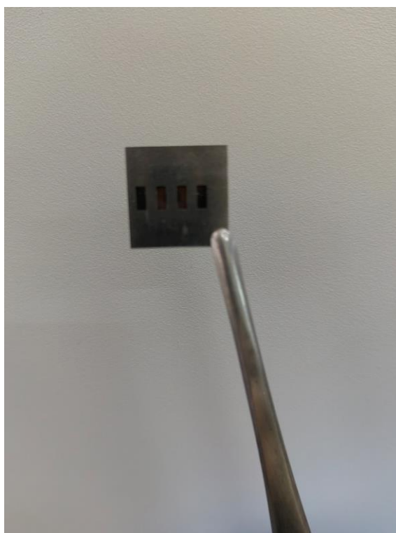
Figure 4. Photograph of the All Inorganic Perovskite Tandem solar cell and Mask
