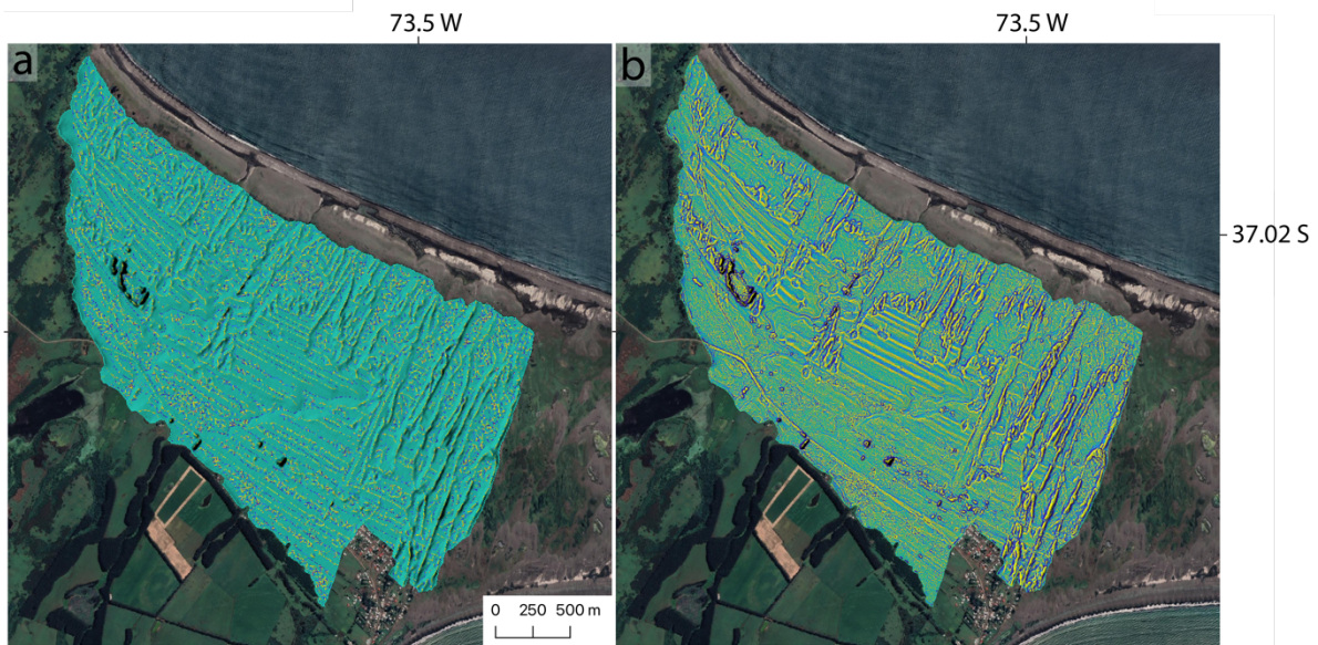
Figure S1. a) Contour curvature of the coastal plain digital elevation model. Note ridge crest in yellow and swales in blue. b) Profile curvature of the coastal plain digital elevation model. Note clear surface geomorphic expression of ridge crests. NNE-SSW oriented crests correspond to elongated dunes.
