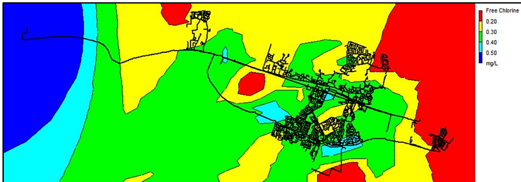
Figure 12. Contour plot of chlorine concentration when the sources' free chlorine concentration was assumed to be 0.6 ppm.
