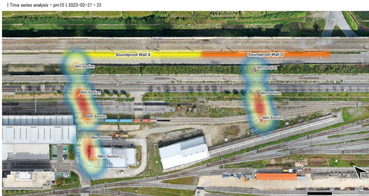
Fig. 4. Effect of fine dust on distance depending on the presence or absence of a soundproof wall.
