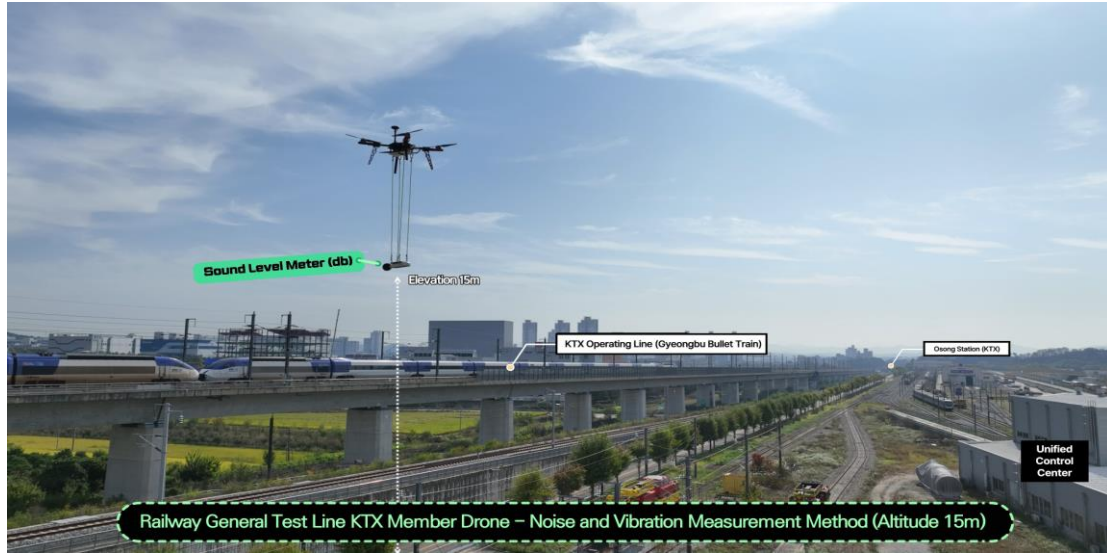
Fig. 9. Method of attaching a noise meter to a drone related to environmental impact assessment of railway noise.
