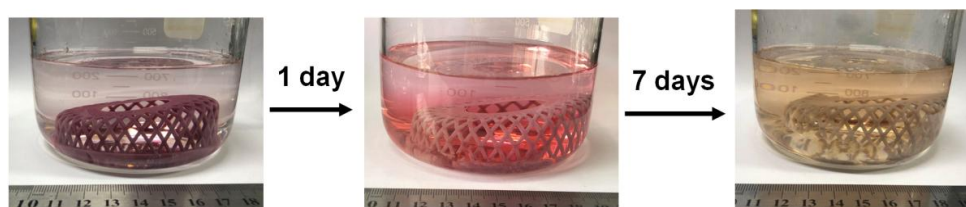
Supplementary Figure 6. Photos of a printed commercial thermoset object immersed in DMF.
