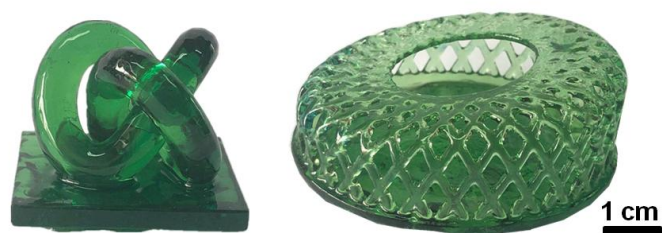
Supplementary Figure 11. DLP printed objects using the recycled resin of dissolving poly(IBOA) in ACMO monomer (3 wt%).
