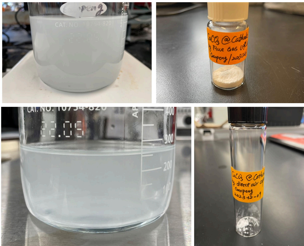
Supplementary Figure 4: Photographs of the catholyte (left) and CaCO 3 solid (right) after electrolysis at 100 mA cm -2 in the presence of the simulated flue gas (10% CO 2 , 90 % N 2 ) (top panel), and air (bottom panel).
