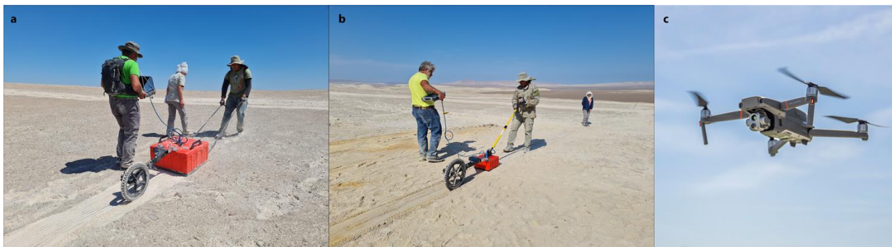
Figure S7. Survey instrumentation. (a) SIR 4000 GSSI system equipped with a 200 MHz antenna and survey wheel. (b) Same system equipped with a 400 MHz antenna. (c) DJI Mavic 2 Enterprise Dual drone.
