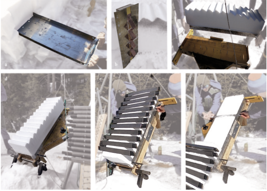
Fig. S4 | Experimental procedure. a Aluminum sled pushed into the snowpack to facilitate the extraction of the snow column of interest. b Profiling device used to serrate the slab's top surface to support the addition of weights. c Placement of snowpack-sled assembly onto the tilting rig with guiding plates on the sides and the bottom edge to ensure alignment. Screws punch into the substratum to prevent sliding. d Assembly tilted to final inclination before addition of weights. e Weak-layer cut introduced with the back of a snow saw by two people ensuring parallel movement through the weak layer. f Slab sliding after unstable propagation of the introduced crack. The cut length is recorded from the end of the saw to the end of the slab.
