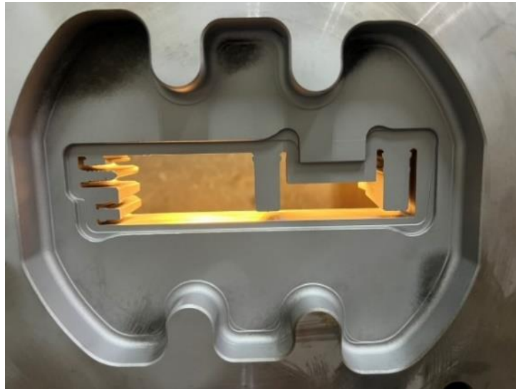
Figure 24. Lower die for the major revision design.
