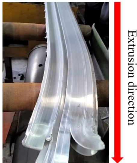
Figure 13. Front end of extruded product after first extrusion test.
