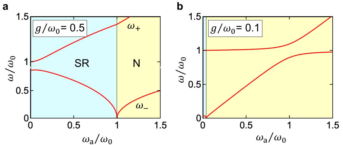
**Fig. S1. Occurrence of the superradiant phase transition at finite detuning.** **a, b,** Normalized frequencies of the upper-polariton ( $\omega_+$ ) and lower-polariton ( $\omega_-$ ) modes as a function of  $\omega_a/\omega_0$  calculated using the Dicke model without the  $A^2$  term with  $g/\omega_0 = 0.5$  (**a**) and with  $g/\omega_0 = 0.1$  (**b**).
