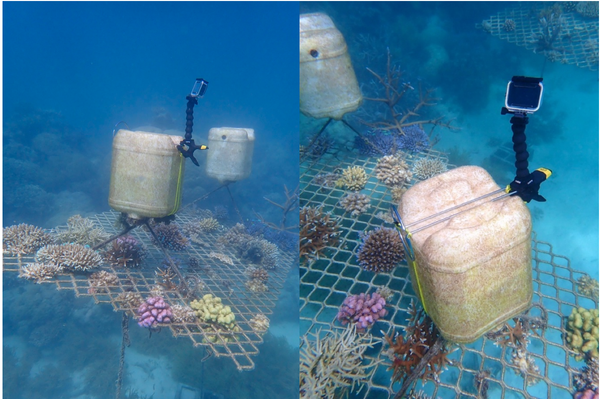
Fig S3 Fish video survey setup consisting of a GoPro Hero 8 camera attached to a GoPro Jaws: Flex Clamp and clipped onto a toilet roll holder made of chrome plated iron wire (50cm (H) x 14cm (Diameter)). Roll holders are fixed on top of nursery floats using nylon rope so that cameras were high enough to capture the entirety of a nursery frame. Photo credit: Gemma M Gillette
