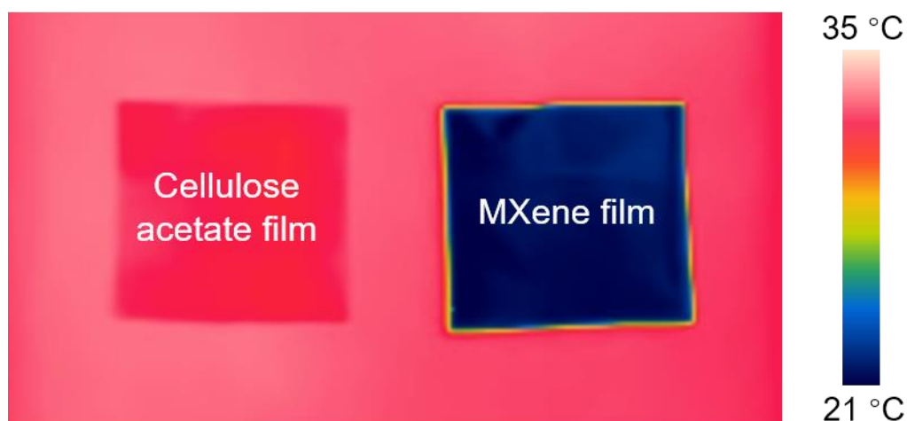
Supplementary Fig. 7. IR photograph of the CA and MXene films on a simulated skin heater.
