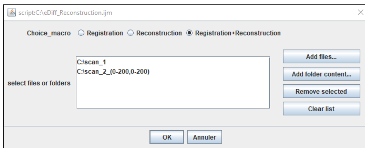
Figure S 9 Interface of eDiff_Reconstruction ImageJ (Fiji) script: choosing a working mode and folders containing the 4D-STEM datasets as an image sequence.
