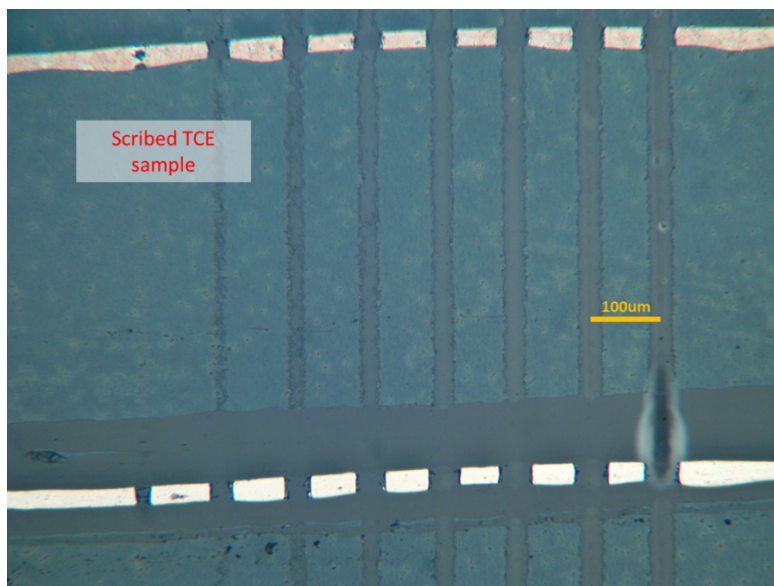
Fig. S5: Laser scribed hybrid TCE sample.
