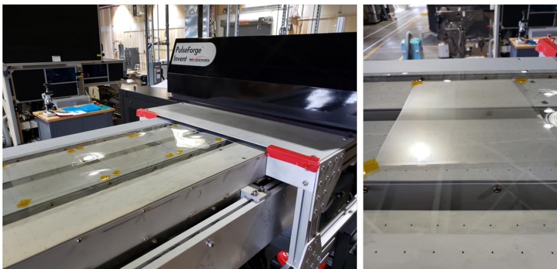
Fig. S4: Images of hybrid TCEs just after being conveyed through the R2R photonic curing tool. The flash lamp is enclosed in the black box, labeled PulseForge Invent, in the left image.
