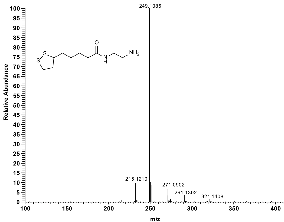
Supplementary Fig. 5 | Mass spectrum (ESI, MeOH) of the lipoic acid-ethylenediamine conjugate which is matched by the peak at 249.1085.
