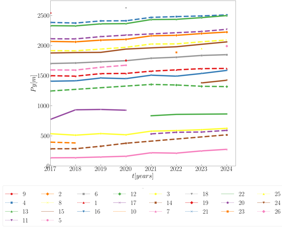
FIG. 35. Time evolution of the longitudinal position P_y of the centroid of bedforms detected in the time sequence of Figs. 27 to 34. The key shows the colors user for each tracked bedform.
