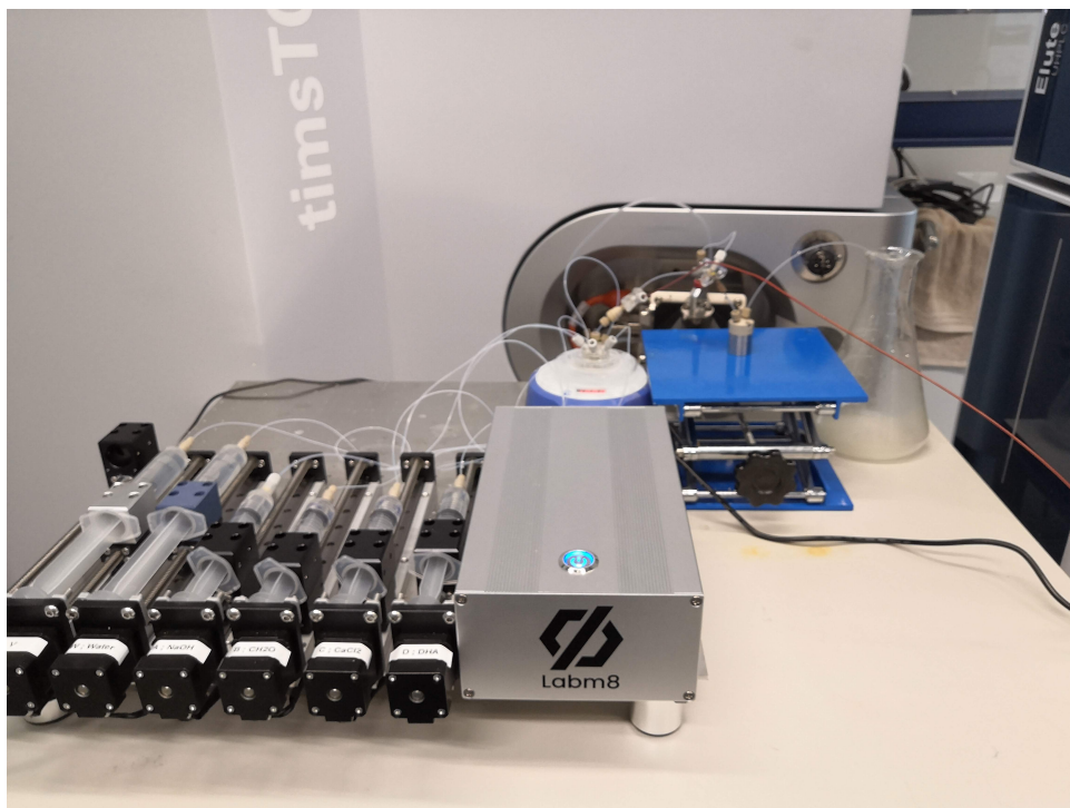
Figure S2: A photograph of the experimental setup. On the left, 6 syringes in a Labm8 pump setup are shown, with labels indicating the syringe content. The flow reactor on top of a stirrer is shown in the middle, with a connection on the right to the back-pressure regulator and waste container. The timsToF instrument is shown in the back.
