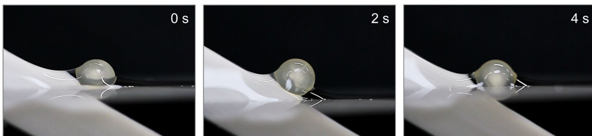
Fig. S3. Sequential images of failed attempts to skim a 3-mm polypropylene (PP) ball using a flat plate tilted at + 60°. For the initial 2s, the PP ball adhered to the plate and lifted before sliding down as the upper water bridge receded (4 s).
