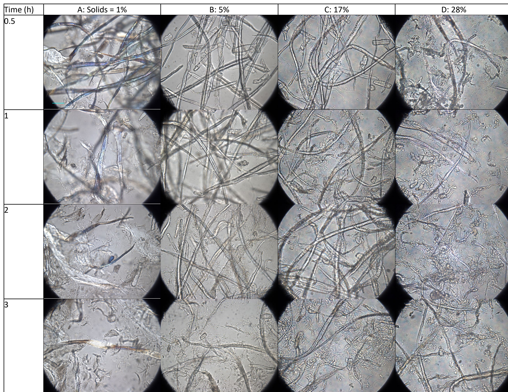
Fig. S3 LM images (40X) of MFC under different solids loadings. Scale bar = 50 \mu m
