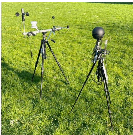
Figure A1.2. Full instrument set up containing HOBOT micro station equipped with thermohygrometer (S-THC-M002), pyranometer (S-LIB-M003) and cup anemometer (S-WSB-M003), Delta OHM weather station equipped with omni-directional hot-wire probe (AP3203) and 15-cm black globe thermometer (TP3275), custom build 4-cm black acrylic globe thermometer.
