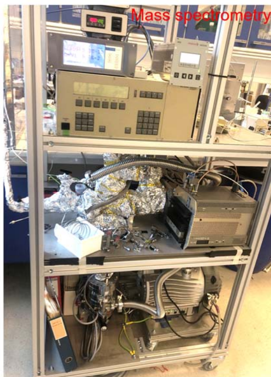
Supplementary Fig. 23 Digital photos of the home-built online mass spectrometry (MS). The MS is placed downstream on the N 2 flow from the cathode side of the flow cell. This allows for operando measurements of the flow cell operation and performance.
