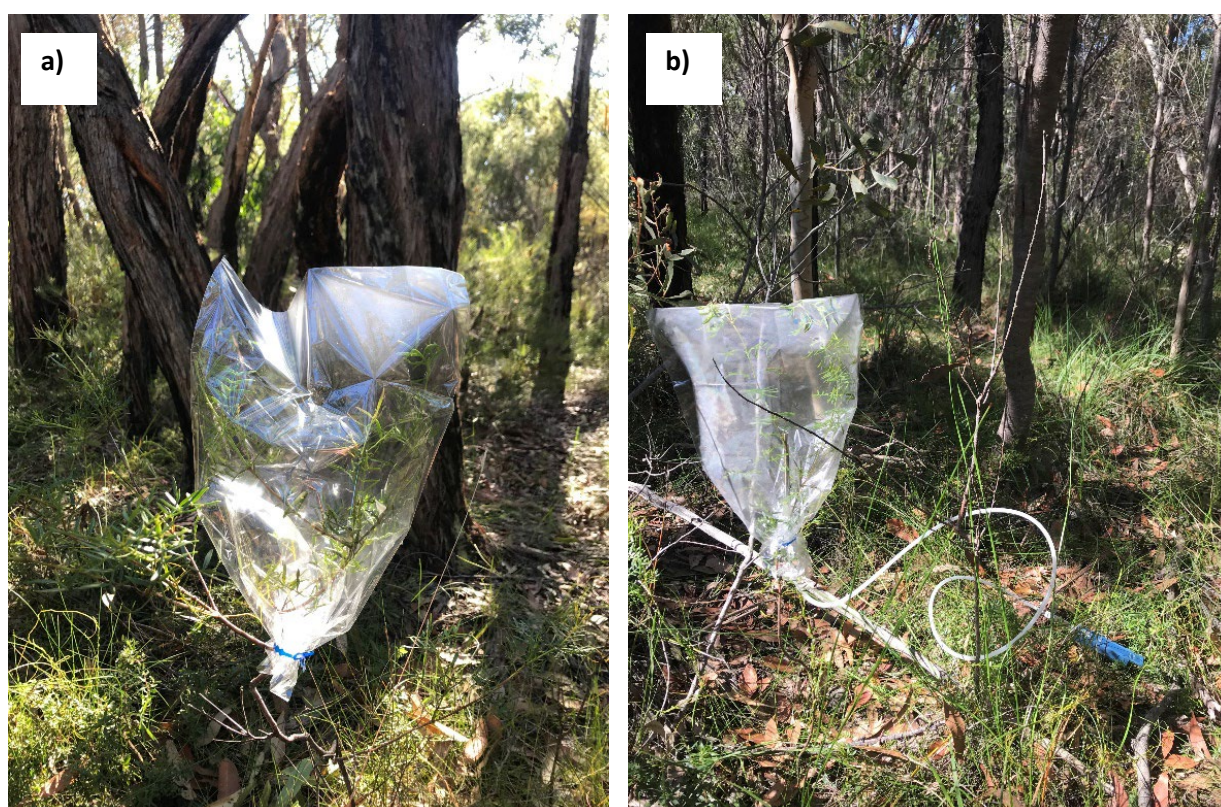
Figure 1. Odour ‘headspace’ sampling of B. pinnata for GC-MA analysis. a) Polyacetate oven bag over a single B. pinnata branch. Odour headspace was allowed to accumulate in the bag for 15 minutes prior to sampling. b) Air was extracted from the bag for 15 minutes through a thermal desorption tube filled with 200 mg of Tenax TA using a PAS500 Personal Air Sampler.
