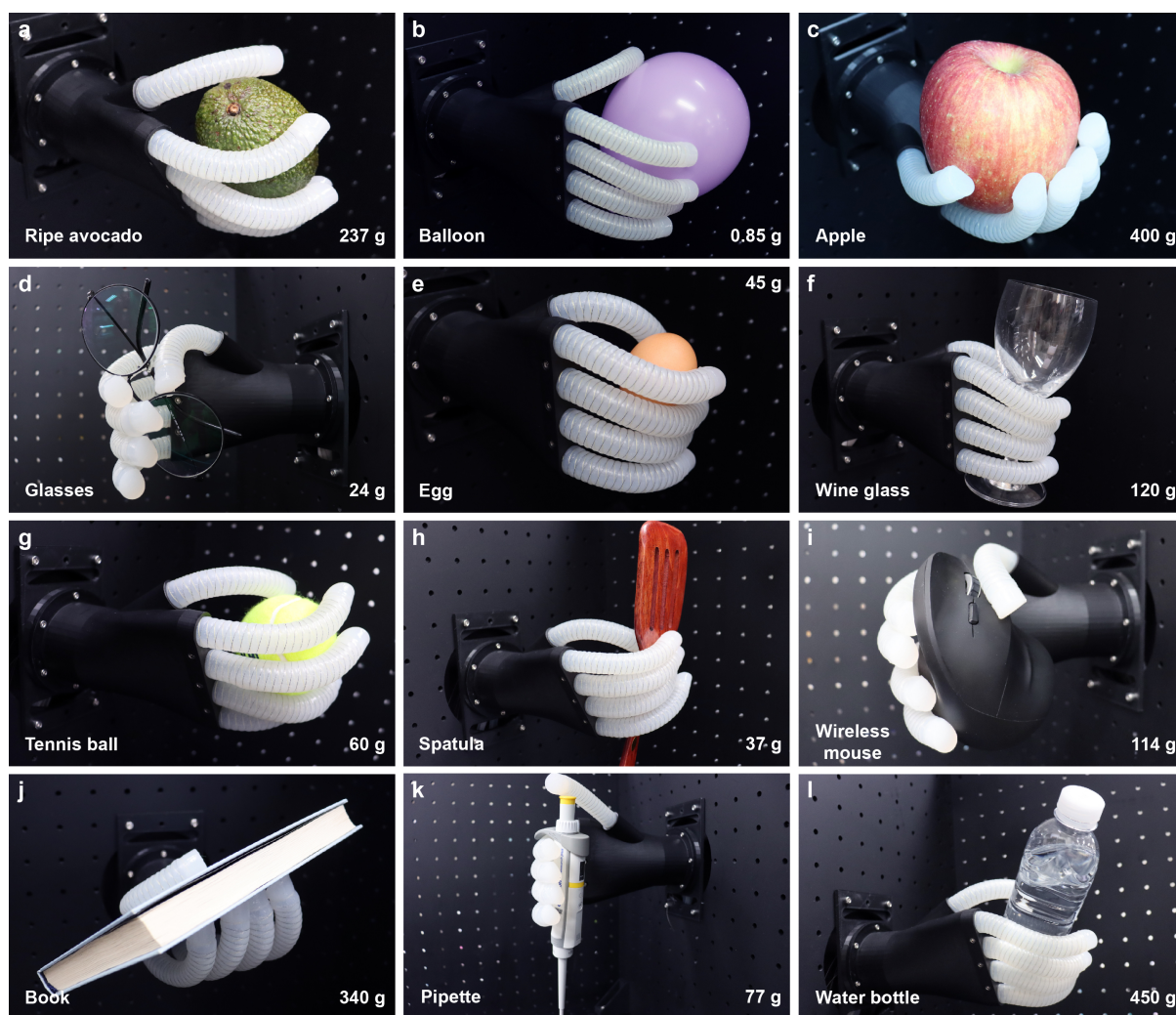
Supplementary Figure 27. Soft prosthetic hand gripping diverse objects. Grasping a (a) ripe avocado, (b) expanded balloon, (c) apple, (d) eyeglasses, (e) egg, (f) wine glass, (g) tennis ball, (h) spatula, (i) wireless mouse, (j) book, (k) pipette, and (l) plastic bottle with water.
