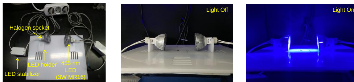
b ■ String-type LED (452 nm) set-up for film curing
