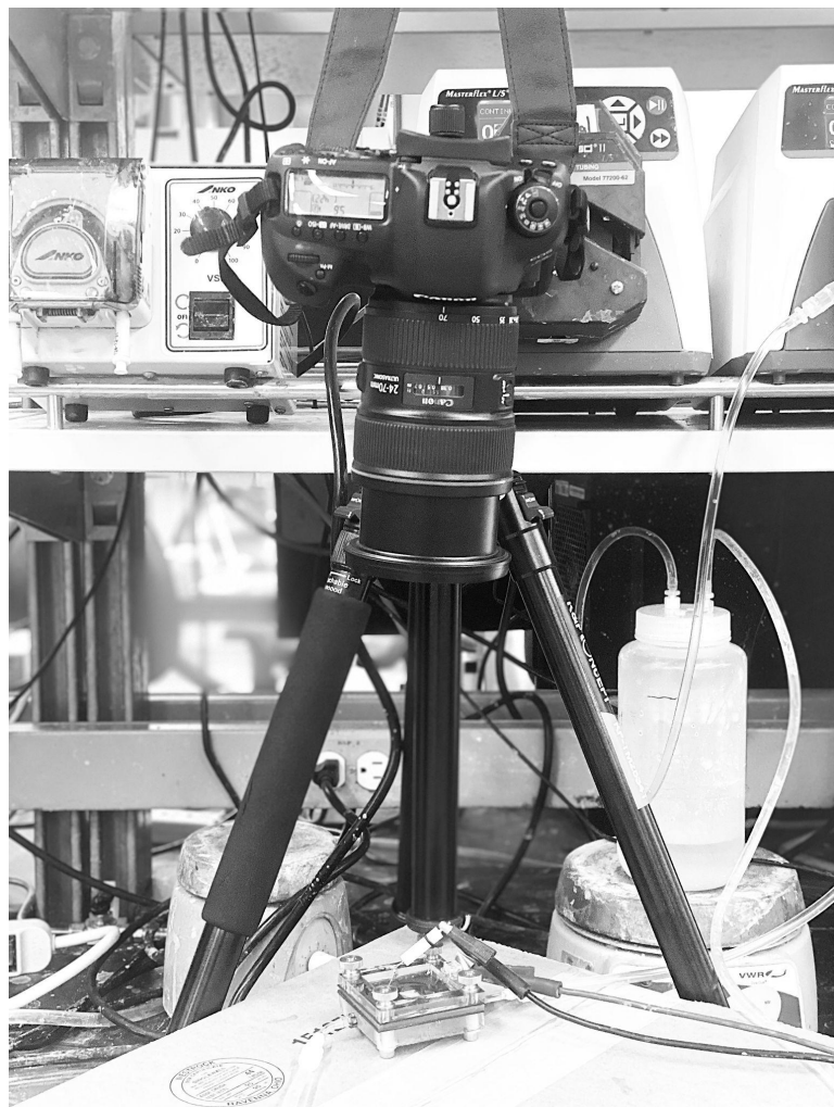
Figure S5. The optical photo of the operando imaging system. The imaging system consisted of a modified two-compartment electrolyser with an open cathode compartment so we could image the CEM through the transparent catholyte with a high-resolution single-lens reflex (SLR) camera fixed above the electrolyser
