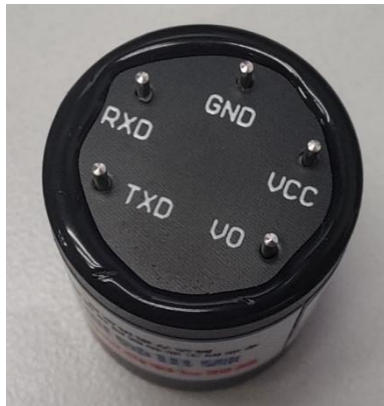
Supplementary Figure 1. Photo of gas sensors used in the dataset establishment.
