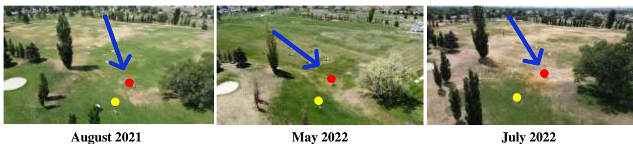
Fig 7. Aerial views of turfgrass and tree canopy on August 01, 2021, May 02, 2022, and July 27, 2022. The eddy covariance flux tower is marked with a red circle, the net radiometer and soil heat flux plates are marked with a yellow circle, and the predominant wind direction is marked with a blue arrow.
