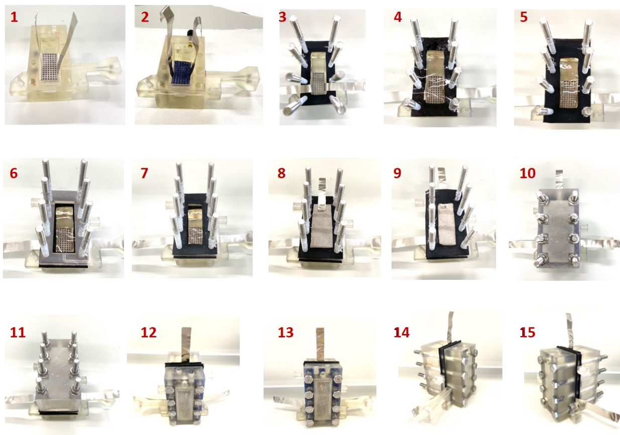
Fig. S17. Schematic of assembling the customized H-cell electrolyzer
