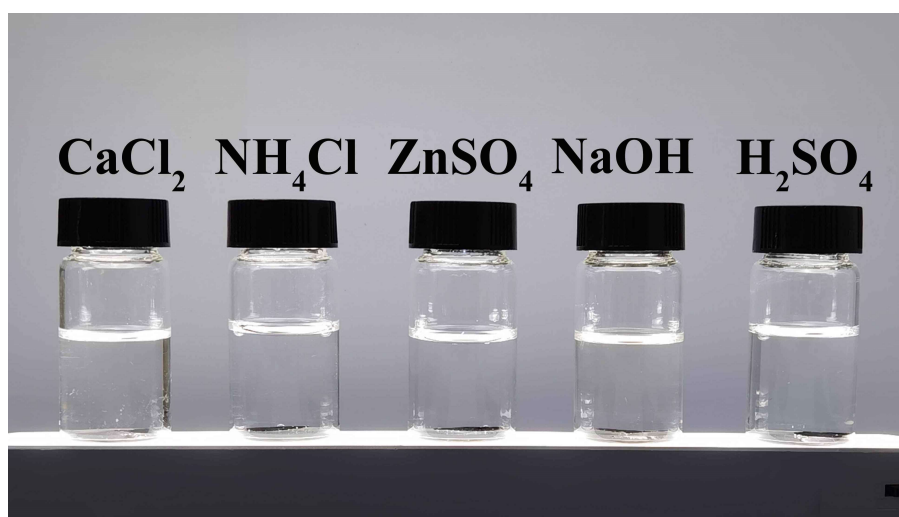
Supplementary Figure 14. Digital photos of the PPHZ electrodes soaked in different aqueous electrolytes without any dissolution after 30 days.
