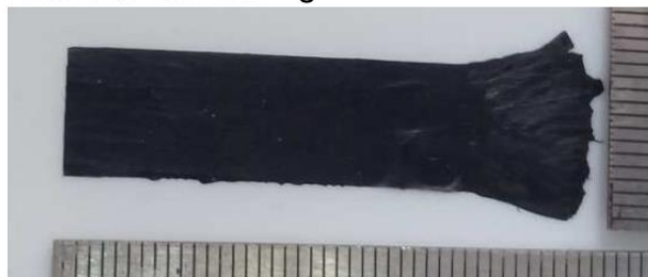
Fig. S9: Optical microscopy images showing the hammering process. It is well revealed that the CNT/PEI film exhibited superior ductility. By hammering the right side of the composite film, both the length and width dimensions could extend by more than 30%.
