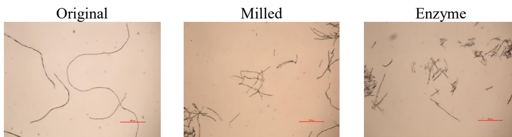
Figure S2. Optical microscopy images of undyed cotton in the original, milled and enzyme treated states. Scale bar 500 μm.
