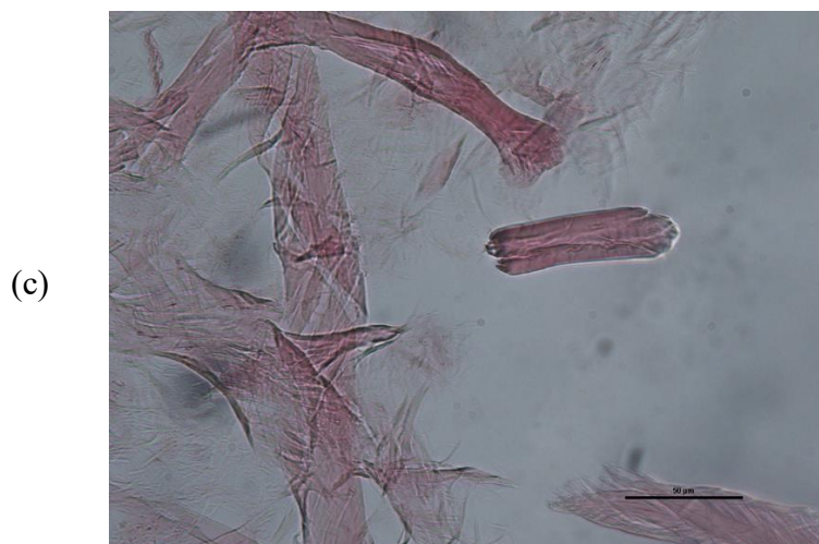
Figure S3. Optical microscopy images of (a) undyed, (b) blue and (c) red cotton fiber fragments resulting from 116-hour treatment in the 2mag mixer with a cellulase dose of 16 FPU/g fabric. Scale bar 50 \mu\text{m} . The less degraded narrow dark red segment in the fiber fragment near the top of (c) and the dark, approximately 50 \mu\text{m} long cylindrical fragment near the center-right of (c), with cracks parallel to its length, are evidence of zones in cotton fibers called “reversals”.
