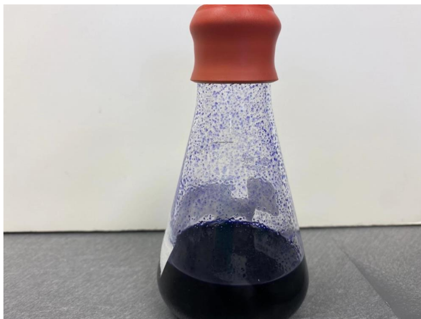
Figure S4. Red cotton dissolved in CED solvent overnight.
