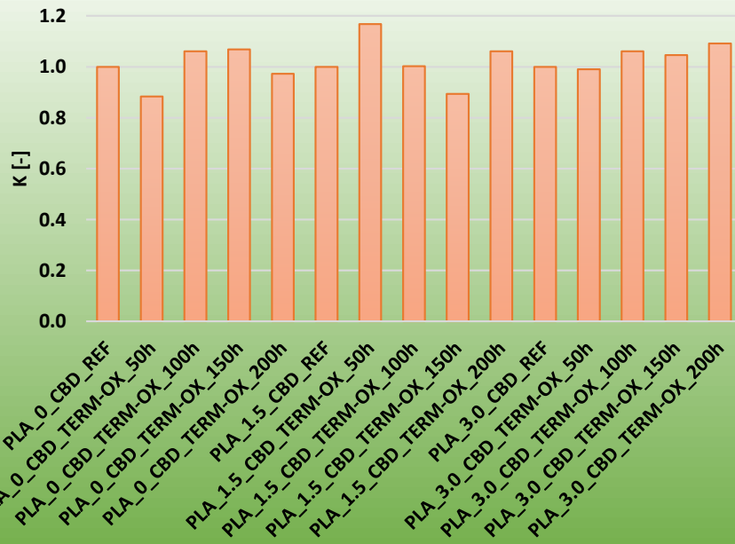
Change in the value of the aging coefficient for PLA samples aged thermo-oxidatively
