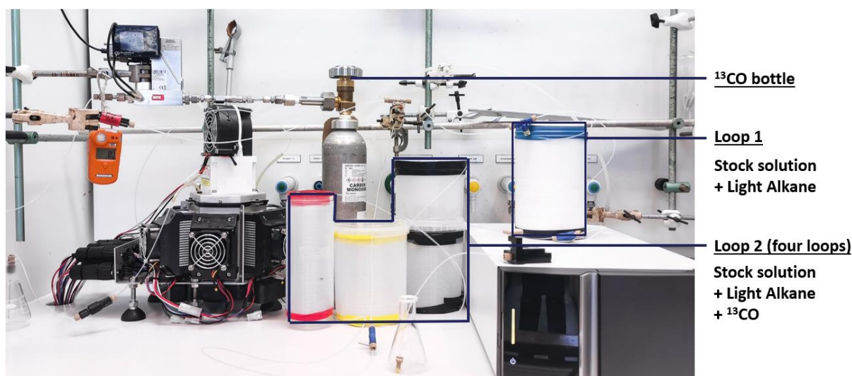
Figure S14: Setup for isotopic labeling experiment of a light alkane using ^{13}\text{CO} . Picture is taken during second loop filling: a gas-liquid mixture of stock solution and light alkane gas (in loop 1) are combined with a gas stream of ^{13}\text{CO} (in loop 2). See protocol gas-gas-liquid reaction for a schematic representation.
