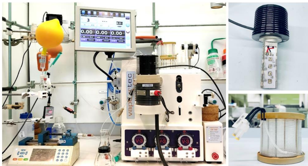
Figure S2: Overview of Vapourtec Setup and detail of LEDs and PFA reactor coil (1.3 mm ID, 1.6 mm OD, 10 mL).
