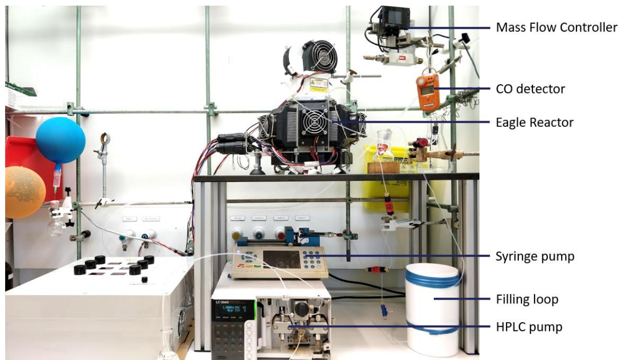
Figure S4: Overview of Setup with Signify Eagle Reactor.
