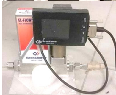
Mass Flow Controller (Bronkhorst EL-FLOW)
