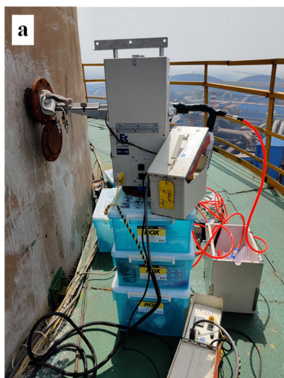
Supplementary Figure 15. Photographs of the sampling systems employed at the typical stack inlets in the iron and steel industry (a), power industry (b), and cement industry (c).
