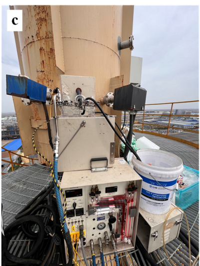
Supplementary Figure 15. Photographs of the sampling systems employed at the typical stack inlets in the iron and steel industry (a), power industry (b), and cement industry (c).
