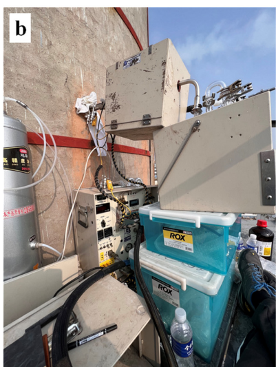
Supplementary Figure 15. Photographs of the sampling systems employed at the typical stack inlets in the iron and steel industry (a), power industry (b), and cement industry (c).
