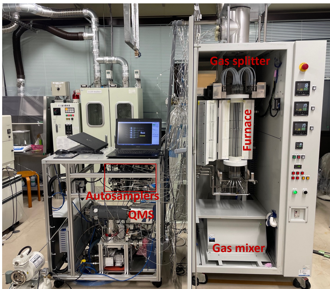
Figure S2: High-throughput screening instrument used for catalyst evaluation
