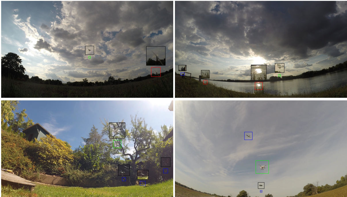
Figure 10. Samples of SAirNet detection results from different videos in the Drone-vs-Bird dataset. The green, blue and red boxes indicate Case 1, Case 2 and Case 3 (described in Section 4.2), respectively.
