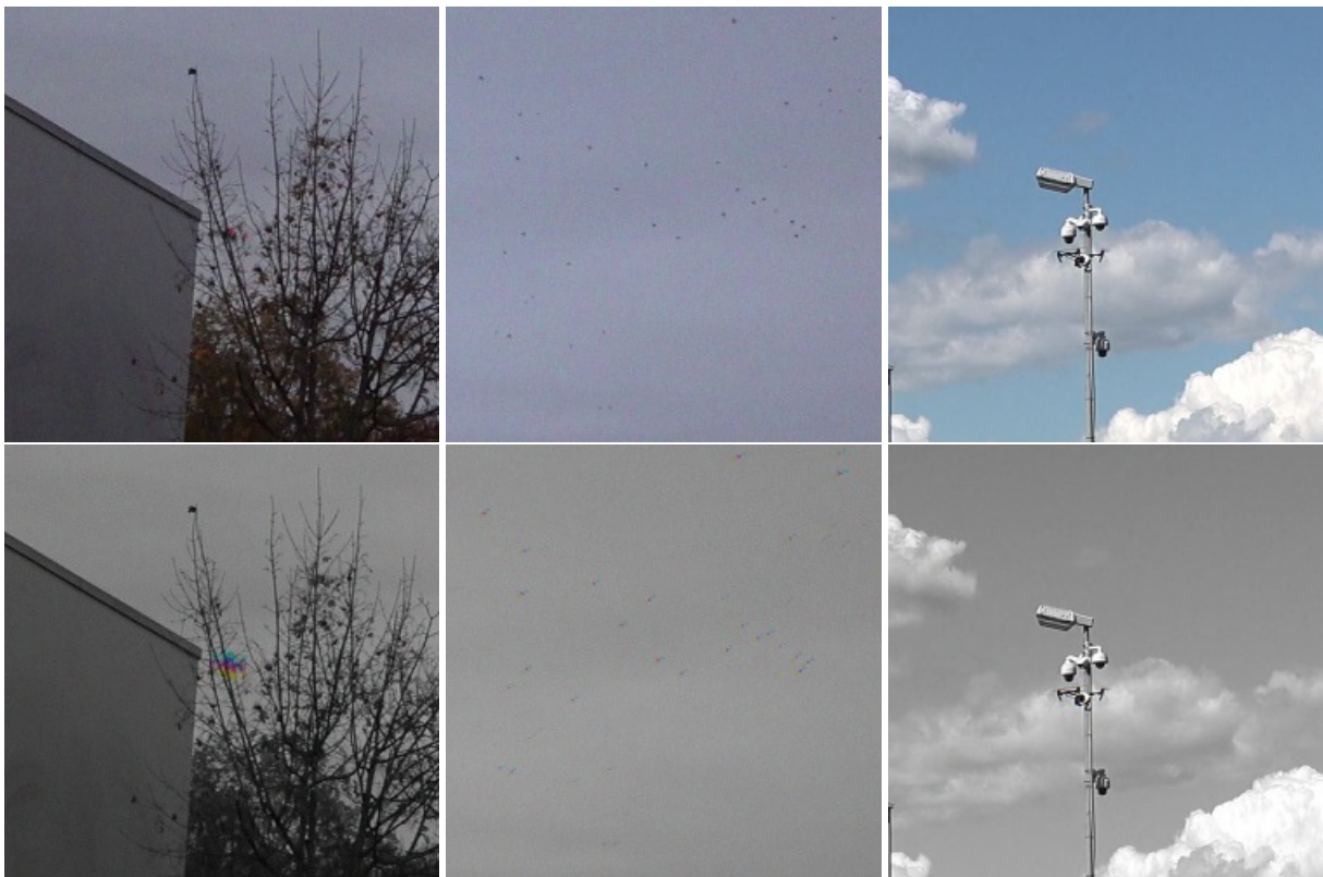
Figure 12. Samples of color images (top) and motion images (bottom), which are an input of SAirNet. Static objects are monochrome, whereas moving objects are chromatic.
