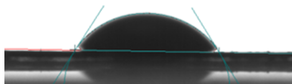
Figure S2. The water contact angle on the graphene/agar/silk fibroin nanocomposite film.
