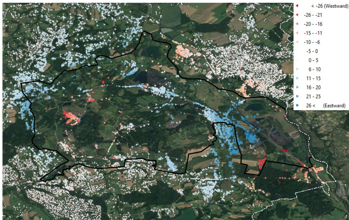
Fig. S4 | Horizontal terrain movement for Poho mining area in Ostrava “follower city”.
