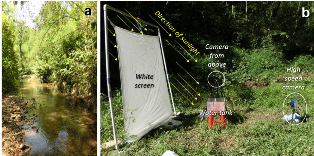
Fig. S3. Field methods. a) Study site in the natural habitat of the giant water strider in the Pumat National Park area. b) Experimental setup used in the field to obtain high-speed movies of jumping giant water striders. A water strider was put in a transparent water tank. Jumping was triggered by poking the insect gently from under water using a hook-shaped wire. Battery-operated high-speed camera (TS 1000) was used to film the jump, while standard camcorder filmed it from above to provide information about distance of the insect to the front wall of the tank (this distance was crucial to translate pixel coordinates into centimeters). A white sheet of fabric spread behind the water tank appropriately located with regard to the direction of sun light was used as a background. For some jumps, Sony RX10-III was used instead of the TS 1000.
