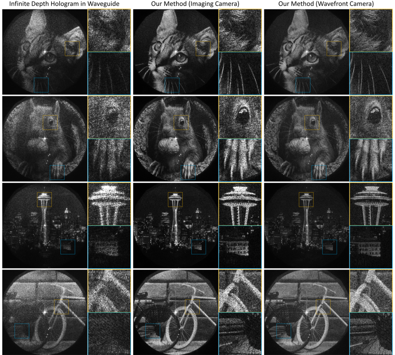
Figure S4. Experimental results of waveguide holography when the images are displayed at infinity (0 D). The insets correspond to 1.3 degree of field of view. Our model improves the image quality significantly even when the image is displayed at the infinity depth, where there is no explicit presence of ghost noise. It demonstrates that our method can overcome the non-idealities in the waveguide display system such as surface aberration and beam clipping effect.
